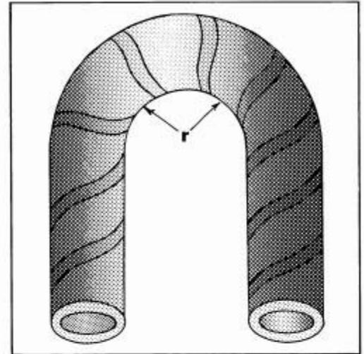
Hose up to 50mm I.D. — 6 times the inside diameter.
